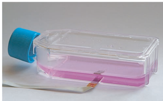
Figure 1. Sensing cell culture flask (SCCF). A sensor chip, comprising oxygen and optional pH and NO sensors, is integrated in a standard cell culture flask.
